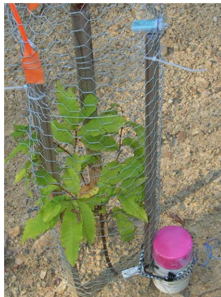
Chestnut seedling with electronic data logger attached. Dataloggers are useful for monitoring temperature, light, and/or moisture conditions for many days at a time and help to determine the environmental conditions that seedlings can tolerate.
